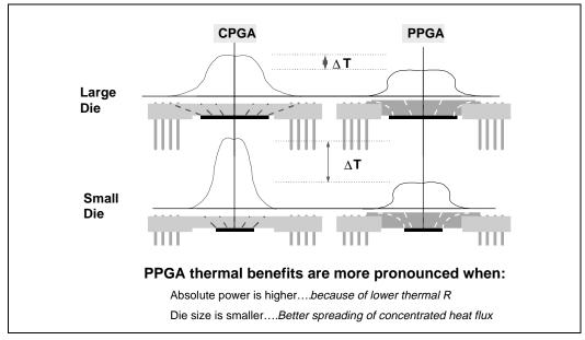
Figure 7. PPGA Has Better Thermal Conduction/Spreading
