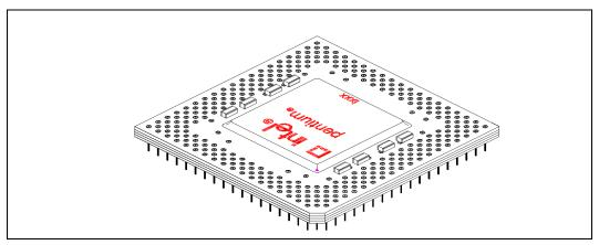
Figure 1. Top View of a PPGA Package
