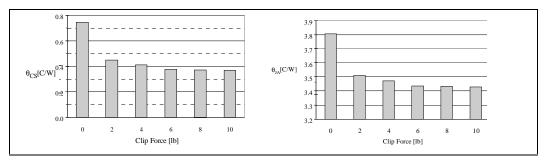
Figure 9. Comparison of  $\theta_{\text{CS}}\,$  and  $\theta_{\text{JA}}$  for Different Clip Forces
