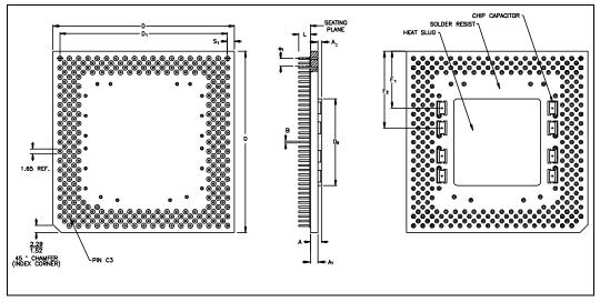
Figure 2. Plastic Pin Grid Array (PPGA) Package Dimensions
