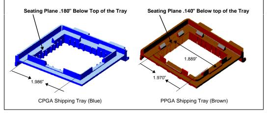
Figure 6. CPGA and PPGA Shipping Trays
