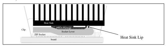
Figure 10. A Heat Sink Design With a Lip
