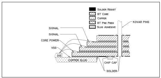
Figure 3. A PPGA Schematic Cross Section
