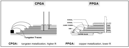
Figure 11. PPGA Has Lower Trace Resistance
