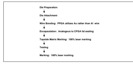
Figure 5. Intel PPGA Assembly Process
