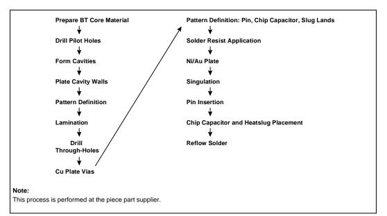
Figure 4. Piece Part Substrate Manufacturing and Lamination Process
